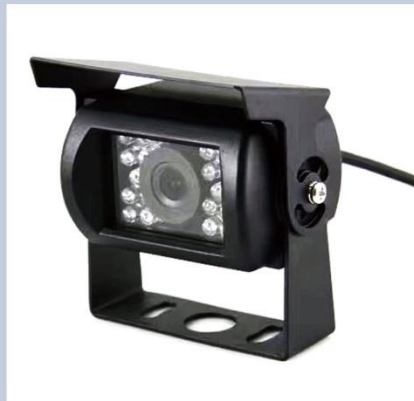
2MP, HD 1920*1080P, IP69K waterproof, 120° wide angle view, Aluminum alloy case
